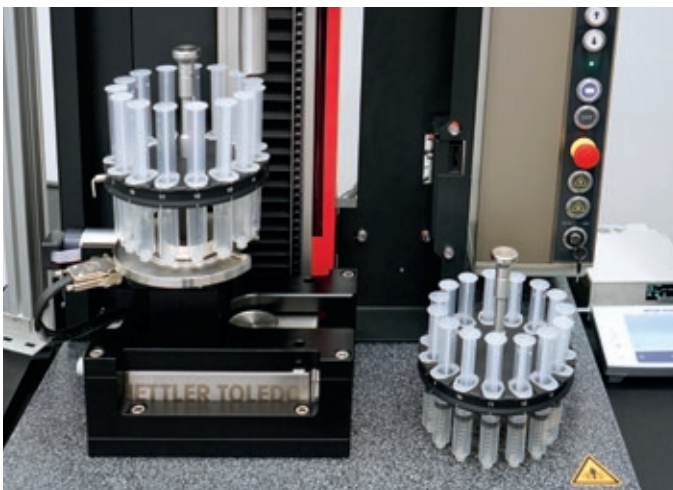
Figure 3: The rotary magazine is used to automatically test 15 syringes one after the other; another magazine can be loaded in parallel.
