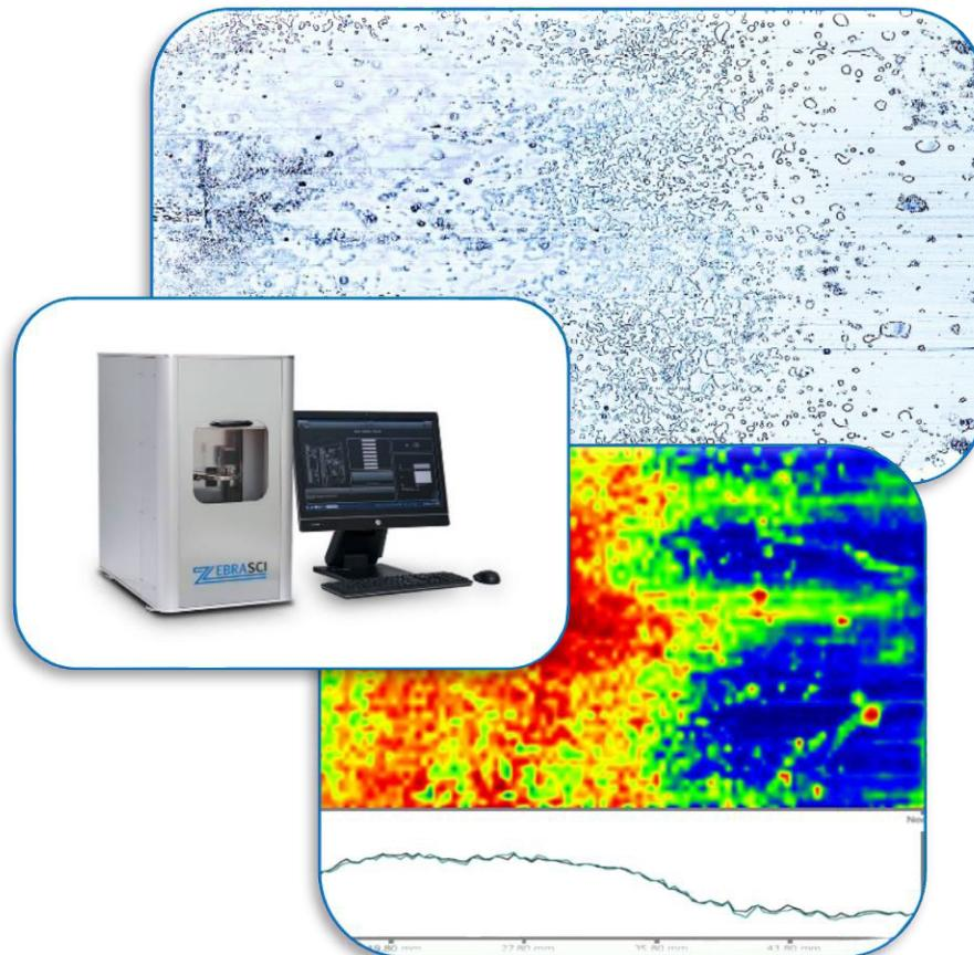
ZebraSci FlexHD Lubricant inspection platform which non-destructively characterizes the amount of container lubrication. This enables one to:
