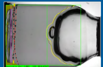
Distinction between particles and bubbles and detection of dark particle
