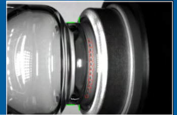
Detection of black particle on stopper
