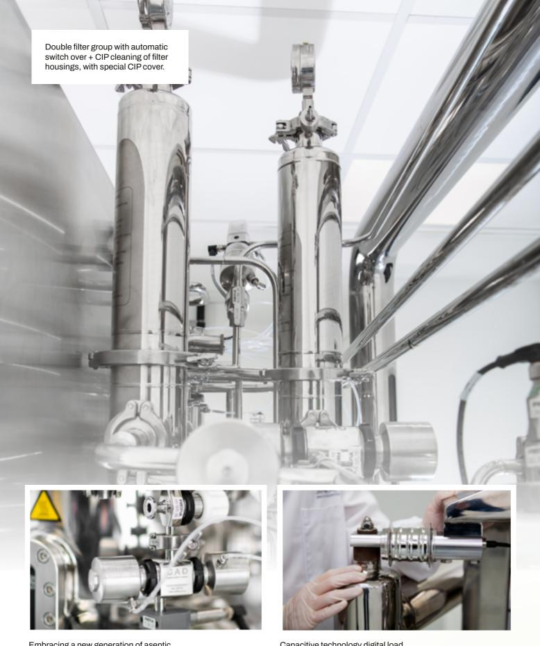
Embracing a new generation of aseptic membrane valves, the Fermi-skid BF50 accelerates CIP cycles, minimizing downtime and maintenance hassles, while at the same time aiding the transition to sustainable production.
