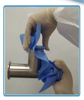
Keystone Cleanroom Products' line of One-Step, Heavy Duty SMS 2-ply wrappers provide an excellent microbial barrier. Ideal for pharmaceutical production applications where two layers are required. Saves time and reduces the amount of autoclave tape.
