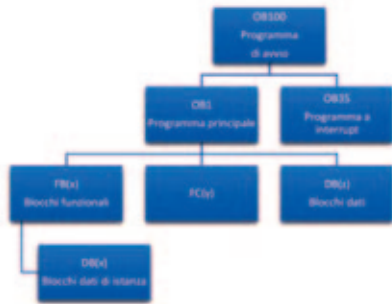
PLC software structure representation
