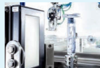
READING AND VERIFICATION OF SERIAL DATA ON A TRANSPARENT LABEL
