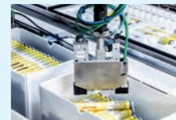
ROBOTIC UNLOADING OF BOXES USING A SCHUBERT 3D CAMERA FOR DETECTING COMPONENT POSITION
