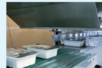
HEAT SEALING OF PLASTIC TUBS WITH FOIL LIDS
