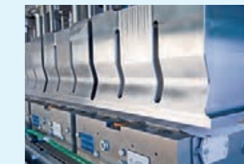
ULTRASONIC SEALING OF BACKING CARDS ONTO BLISTER
