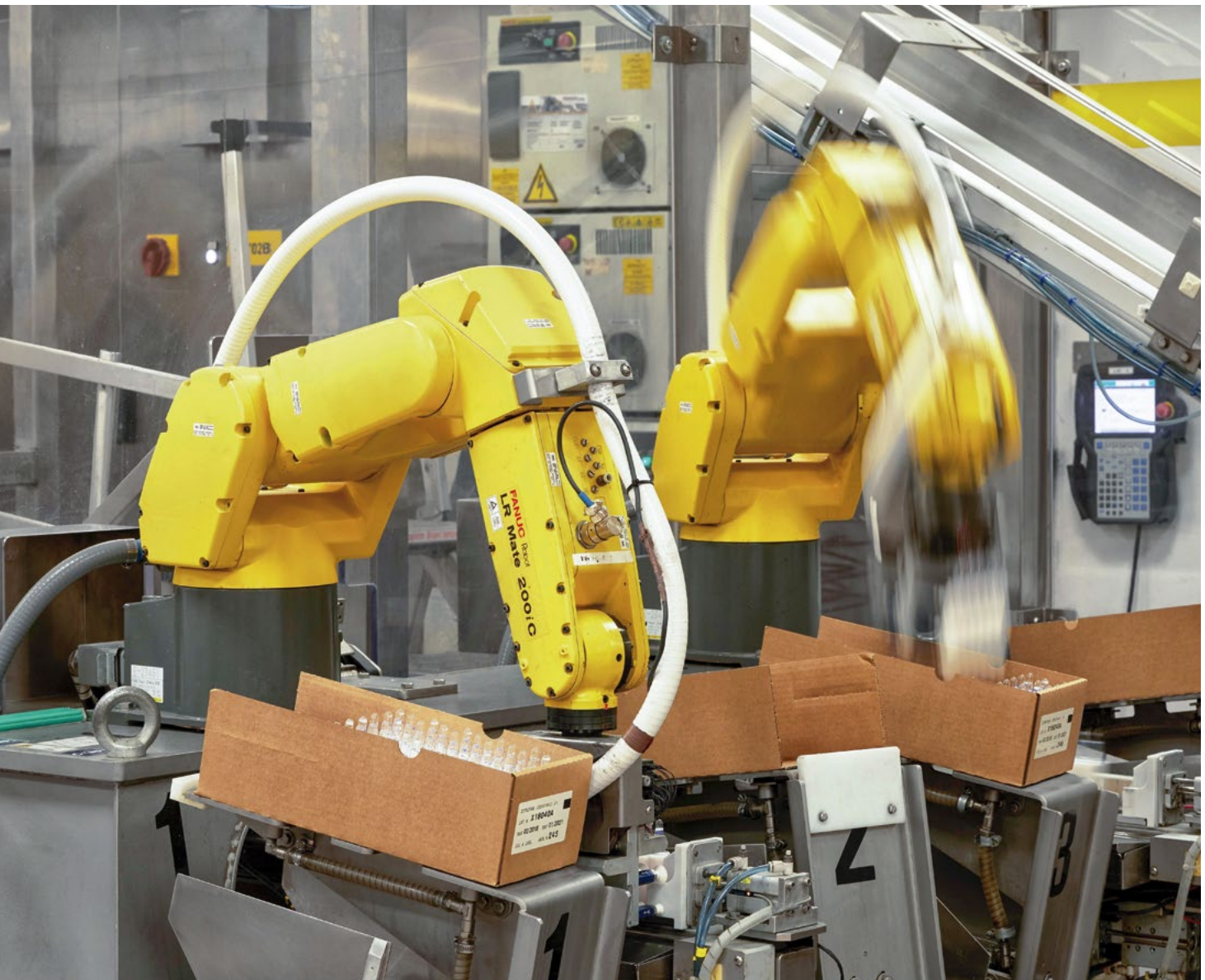
Fully-automated packaging line at CordenPharma Caponago (IT).
