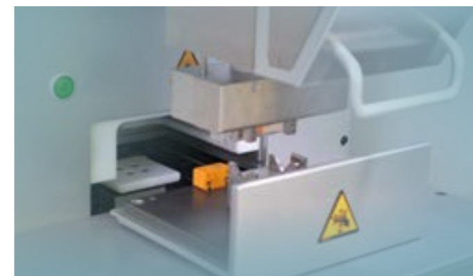
Process integration: laser marking
