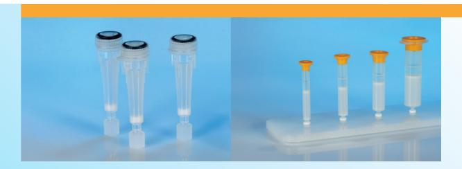
CentriPure Gel Filtration Columns are specifically designed for rapid and efficient removal of small molecules (dyes, salts, biotin, haptens, etc.) from larger proteins, nucleic acids, or nanoparticles, which are simultaneously purified and desalted in a single step.
