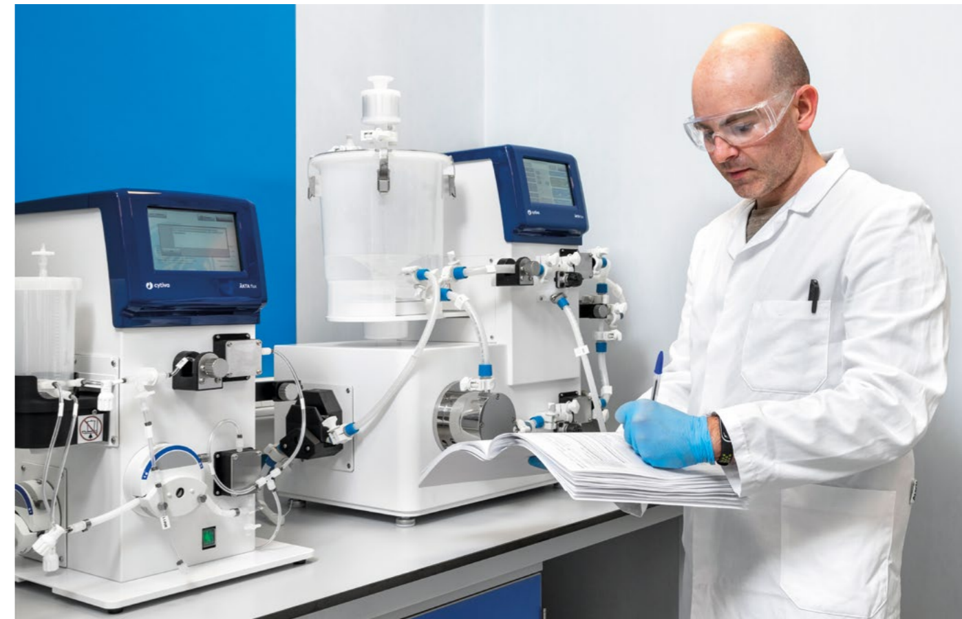
Equipment for ultrafiltration / concentration of LNP-formulated drugs at CordenPharma Caponago (IT).
