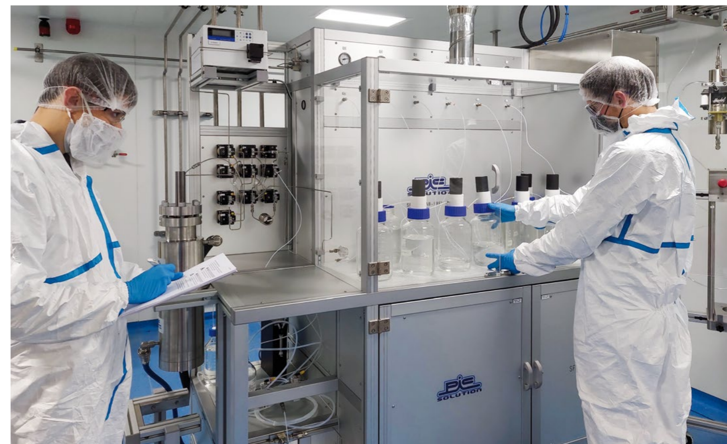
CordenPharma's SFC 1500 (PIC Solution) technology for lipids purification at CordenPharma Chenôve.
