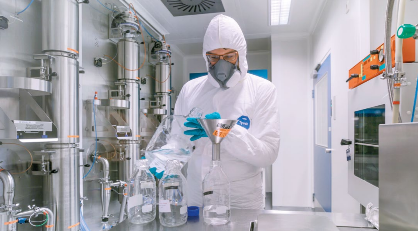
The spray drying process at CordenPharma Brussels (BE) uses an advanced technology to isolate peptides in a very controlled way.
