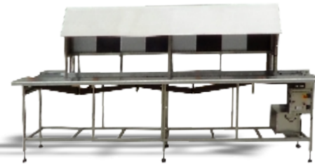
Visual Inspection Conveyor
