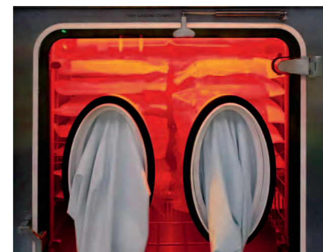
VHP decontamination: Fast Gassing Airlock integrated design for tray offloading
