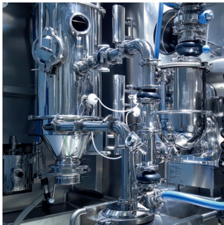
Dry Powder Inhalation Production Isolator integrated MC DecJet® 150
