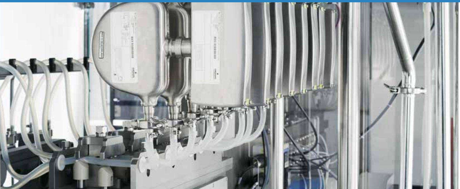
Mass flow dosing system – back view
