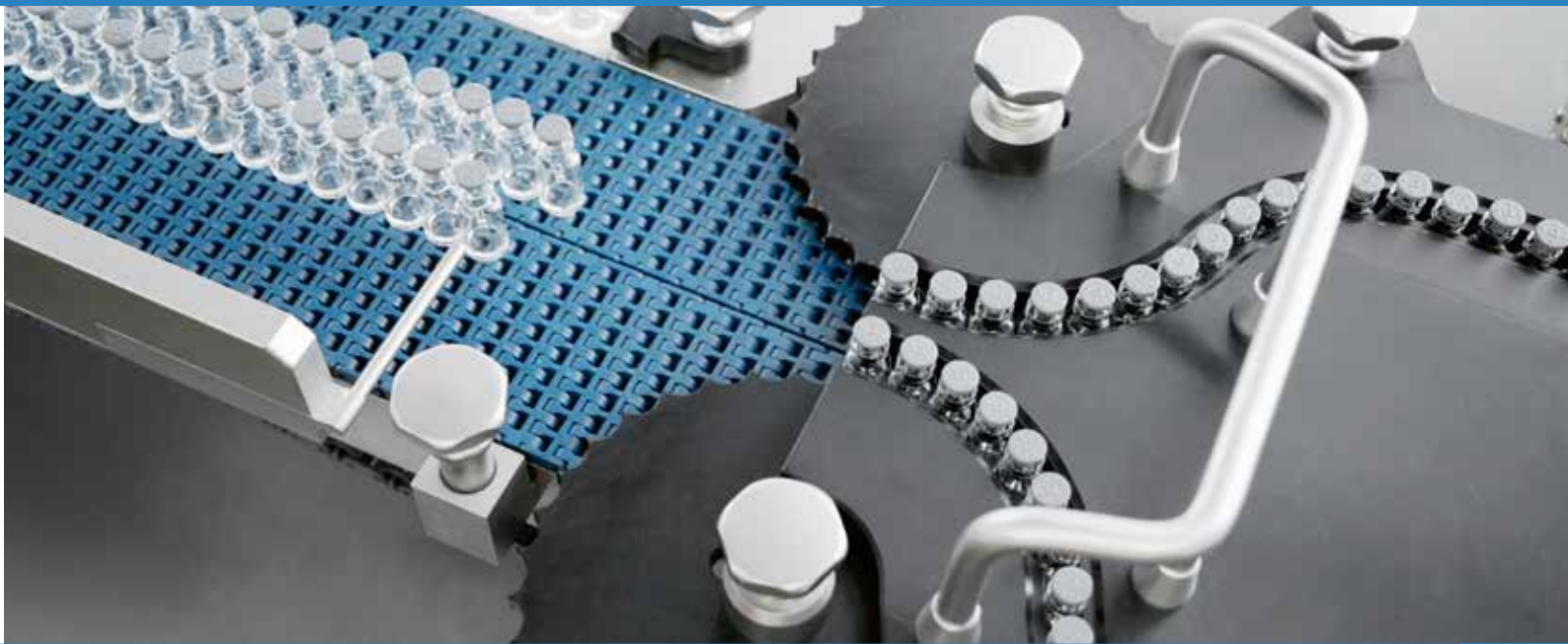
High speed double loading to Freeze Drying with performances up to 600 pcs/min
