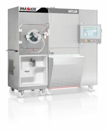
The coating pan processor is equipped with an interchangeable and fully perforated drum.
