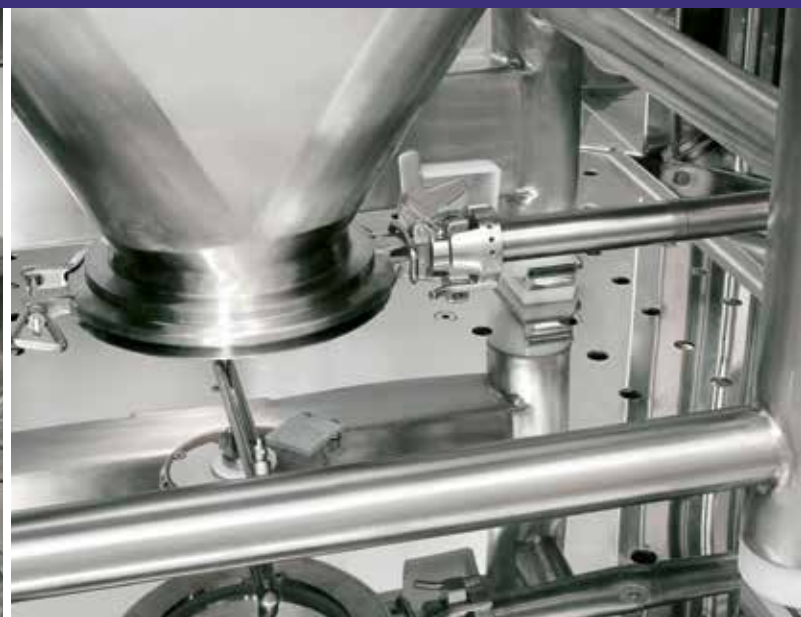
Automatic opening of the lower bin valve
