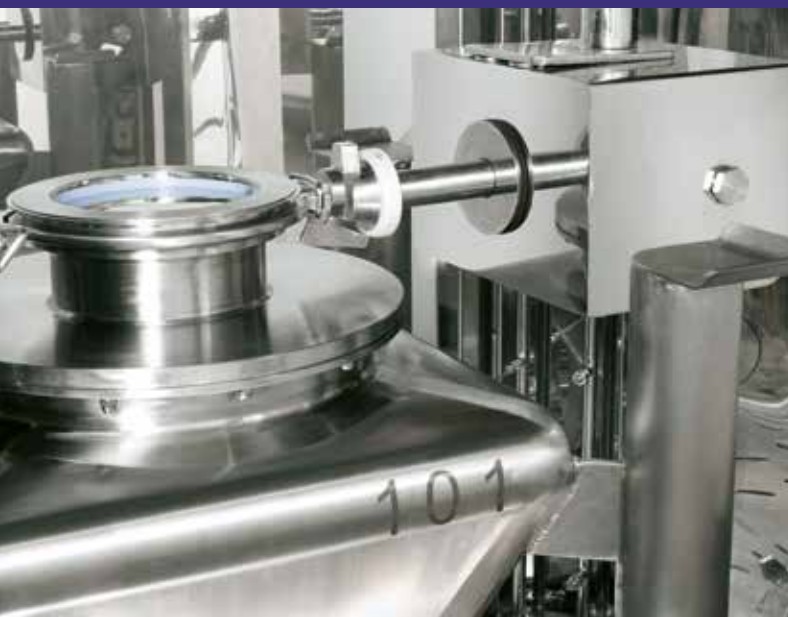
Automatic opening of the upper bin valve
