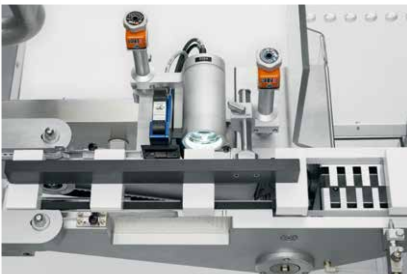
Side printing and camera inspection
