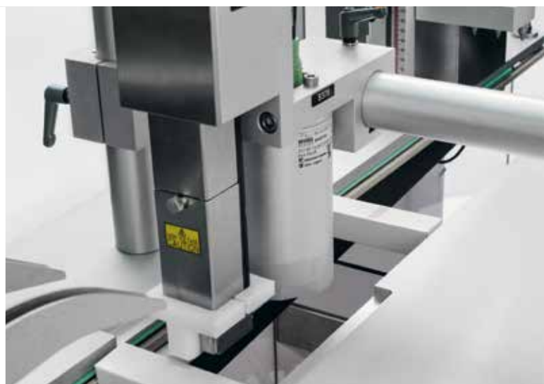
Top printing and camera inspection
