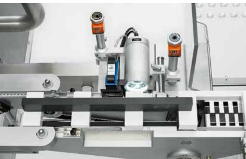
Side printing and camera inspection
