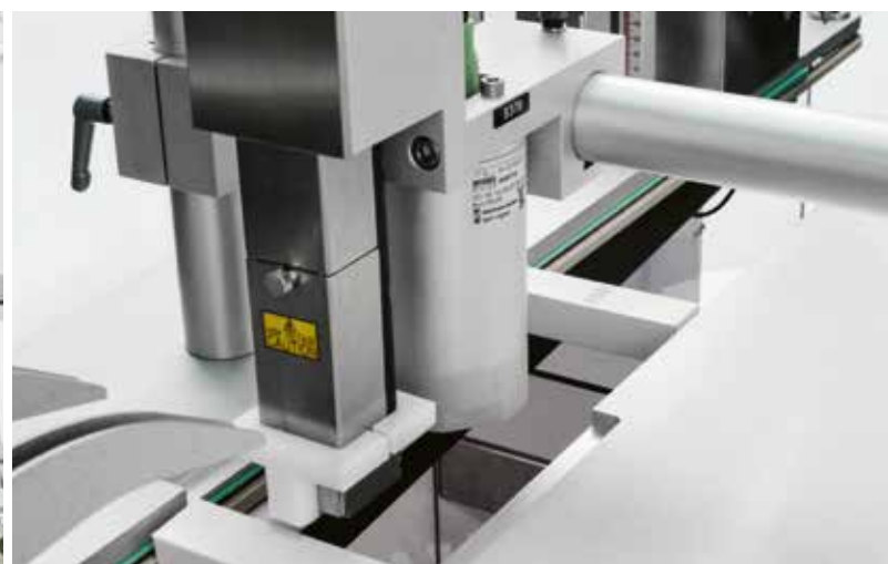
Top printing and camera inspection
