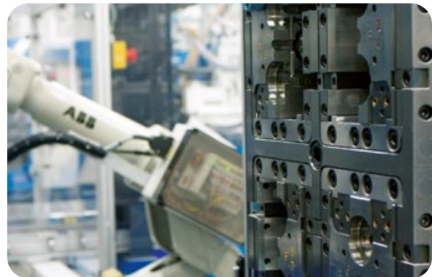
Multi-cavity tool moulding and automated handling systems
