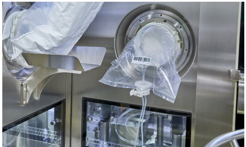
Liquid Transfer DPTE® single-use technology
