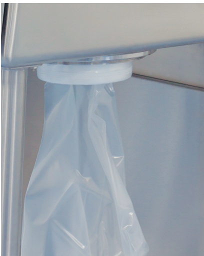
Removal of solids & liquids Samples to QA/Waste via DPTE®
