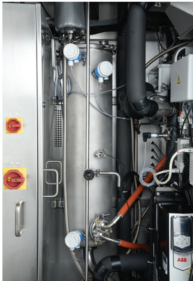
Getinge washer-dryers equipped with SPFR use a two-way, two-valve system to control rinse water delivered to the chamber during the phase. When the recirculation valve is closed, rinse water enters the chamber and pours over the load. The water does not recirculate through the system. This ensures that only the single pass final rinse water is in contact with washed components.
