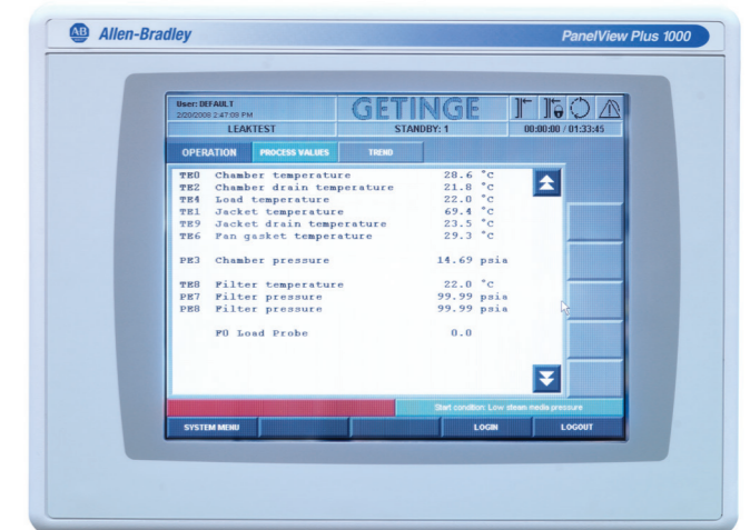
The Allen-Bradley control system incorporates an intuitive touchscreen interface that provides reports, control options and real-time system monitoring.
