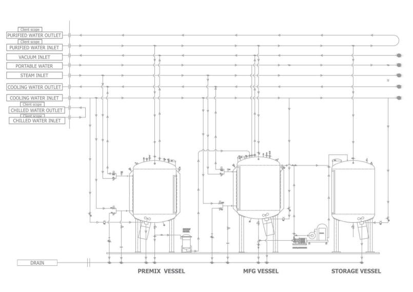
The Liquid Manufacturing Plant is a set of equipment designed for the manufacture of syrups, liquid oral formulations and other water based pharmaceutical products.
